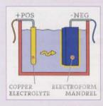
Electroforming is a way of making very accurate metal parts. It is similar to electroplating in that a metal coating is deposited on a special form in an electrolytic solution. The difference is that the coating is thicker so that the form
