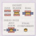
Hydroforming is a way of shaping materials such as aluminium or ultralight steel. The metal is pushed into shape using fluid pressure. For example, to produce components for car bodies, steel tubes are placed inside a mould and high
