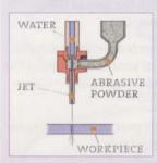
Water jet abrasive cutting uses a high pressure jet of water combined with an abrasive substance to cut through materials. The advantages of this form of cutting are that the jet can be adjusted and the kind of abrasive changed so that
